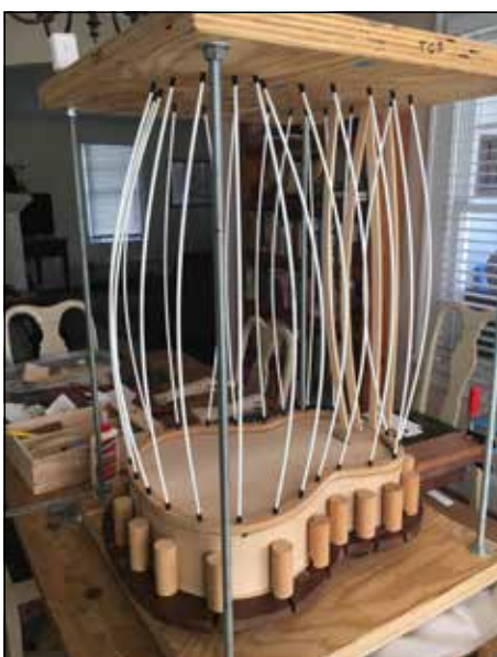
Guitar back, in its jig for gluing (photo by Steve Johnson)
